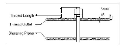
Bolts shall be of such a length that the nut after tightening can be well secured by punching of the exposed thread if required.
